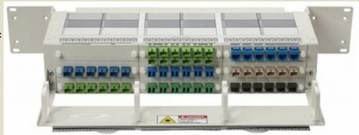
ground locations. Through the use of easily interchangeable panels with industry standard LGX® dimensions, the chassis can handle fiber and copper connections including LC, SC, RJ45 and F81. The HDMC also supports the increasingly popular Multi-fiber Push On (MPO) type connectors.
